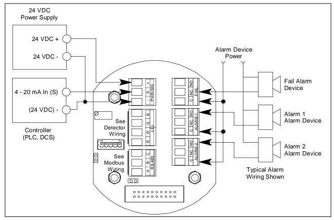
Figure 37: PLC and DCS Device Wiring
