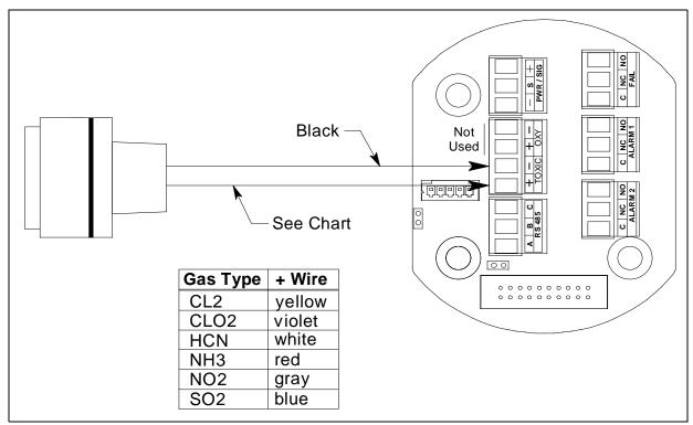
Figure 30: CT-7 Series Toxic Detector Wiring
