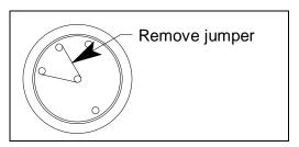
Figure 32: Plug-In Sensor Jumper Removal
