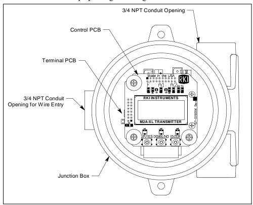
Figure 10: M2A-XL Internal Components
