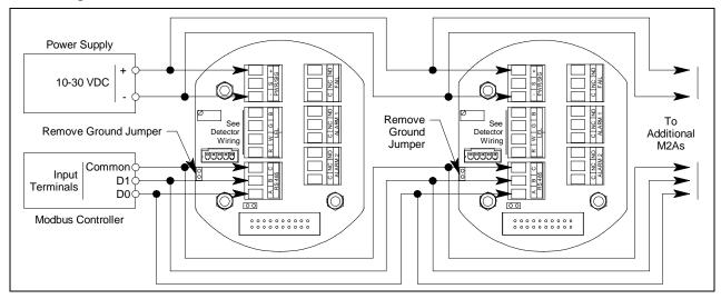
Figure 33: Recommended Modbus Wiring
