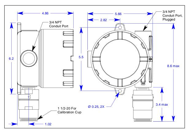
Figure 19: Outline & Mounting Dimensions, H<sub>2</sub>S, CO, HCN, and Oxygen, CSA, Explosion-Proof
