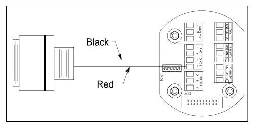
Figure 28: H<sub>2</sub>S/CO Detector Wiring
