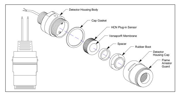
Figure 9: Explosion-Proof CT-7 Series HCN Detector
