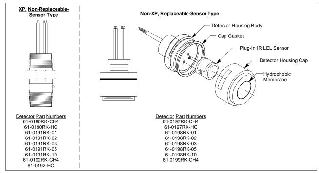
Figure 3: Infrared (IR) Sensors
