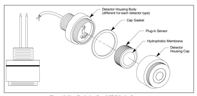
Figure 8: Non-Explosion Proof CT-7 Series Detectors
