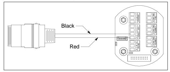
Figure 27: H<sub>2</sub>S/CO/HCN Detector Wiring, CSA
