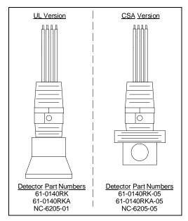
Figure 2: Catalytic Sensors
