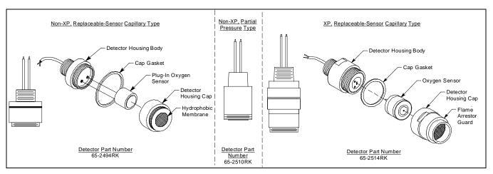
Figure 4: Oxygen Detectors
