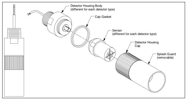
Figure 7: ESM-01 Type Detector
