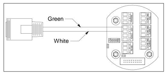
Figure 24: Partial Pressure Oxygen Detector Wiring
