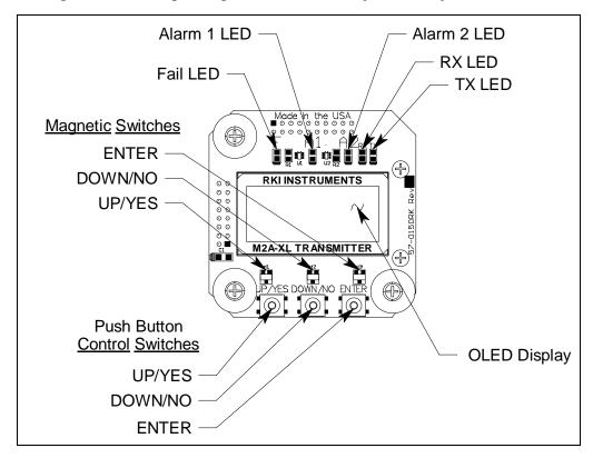
**Figure 13: Control PCB Component Location**
