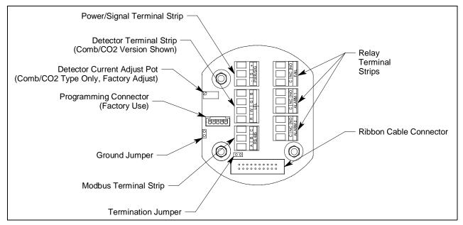
Figure 11: Terminal PCB Component Location
