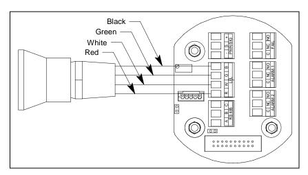
Figure 22: Catalytic LEL and ppm Detector Wiring
