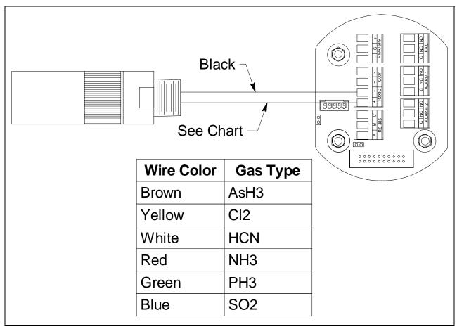
Figure 29: ESM-01 Toxic Detector Wiring
