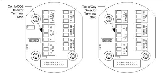
Figure 12: Detector Terminal Strip
