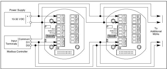
Figure 34: Alternate Modbus Wiring
