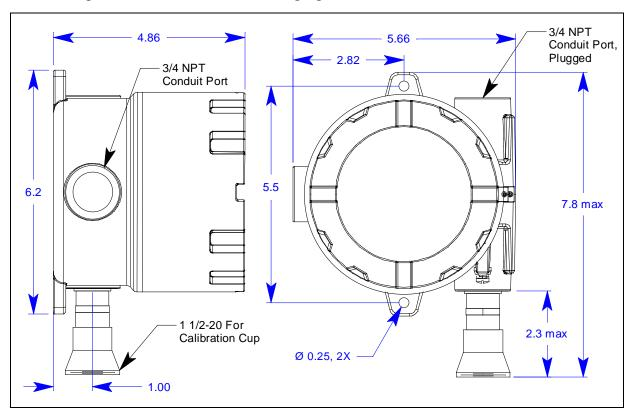
Figure 14: Outline & Mounting Dimensions, Catalytic LEL and ppm, UL Version
